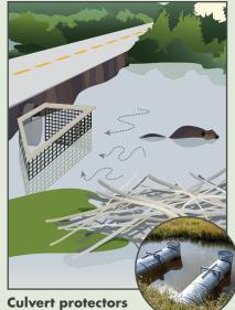
prevent plugged culverts that can cause flooding of roads and other areas.
