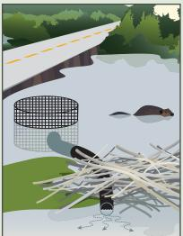
**Pond levellers** mitigate flooding by acting as an overflow valve through a beaver dam, allowing for the pond level to be maintained at a level that prevents flooding but allows beavers to maintain their pond and habitat.
