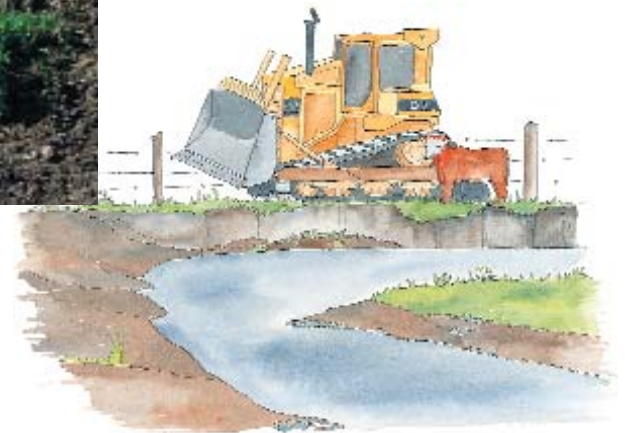
Hoof power can't be underestimated. Cattle exert about 10 times the weight or pressure per unit area as a D9 cat with a blade. The foundation can't withstand this pressure for prolonged periods.
